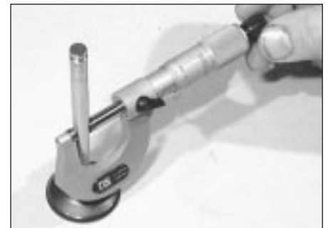
8.17 Measuring the valve stem diameter
