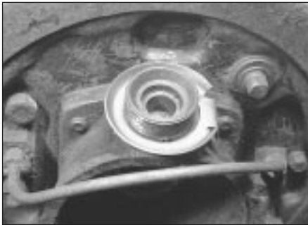
5.11a Fit the lockwasher ...
