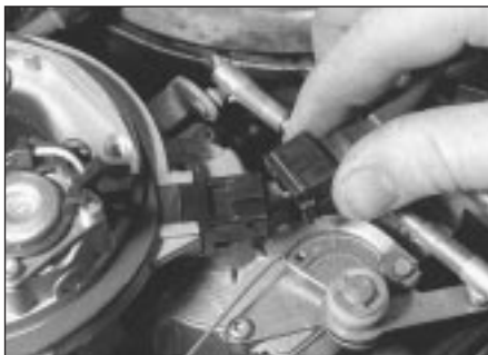
13.12 Disconnecting the injector housing wiring connector
