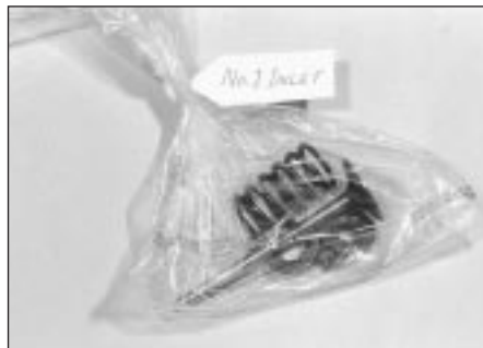
8.6 Keep all valve components together in a labelled plastic bag
