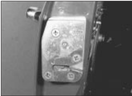
10.4 ... and the door lock retaining screws
