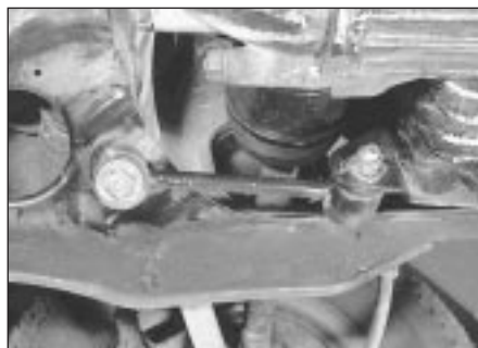
12.30 Lower engine tie-bar attachments
