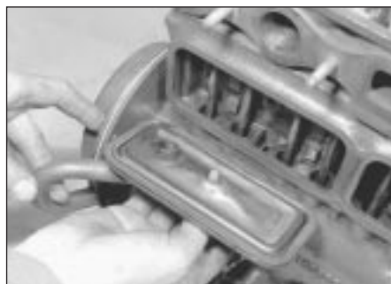
9.1 Removing the tappet side covers
