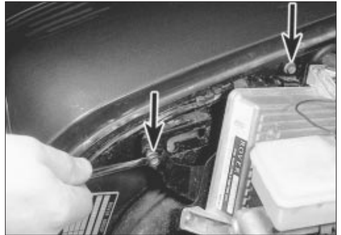
13.30 Undo the ECU mounting bracket-to-wing valance retaining bolts (arrowed) . . .
