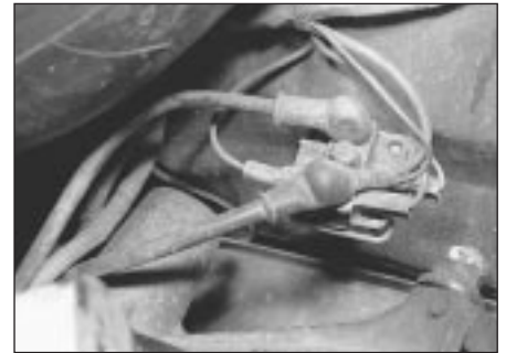
16.2 Electrical connections at the starter solenoid
