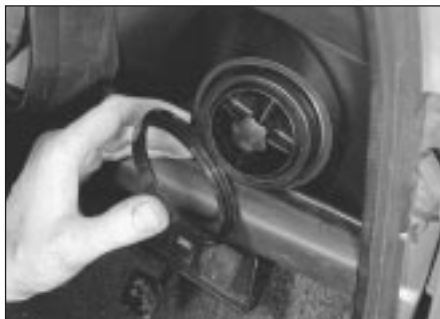
13.1a Unscrew the fresh air vent retaining collar ...
