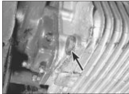
13.3 Engine/transmission oil drain plug (arrowed)
