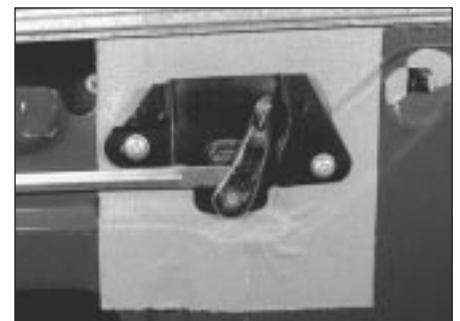
10.3 . . . the interior lock control retaining screws . . .
