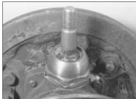
5.12d Bend up the lockwasher ...
