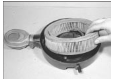
30.6b . . . and lift out the element
