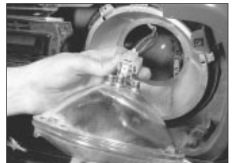
5.5 Detach the electrical connector and lift away the light unit
