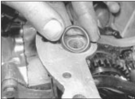
5.26 . . . and a new O-ring to the transmission casing joint face
