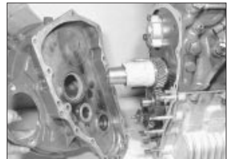
5.35 Refitting the flywheel housing
