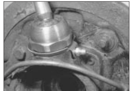
5.12b ... screw in the grease nipple ...
