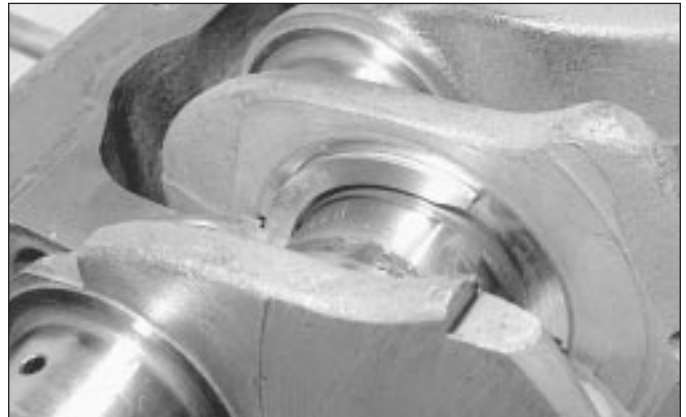
17.19 Refitting the crankshaft thrustwasher upper halves
