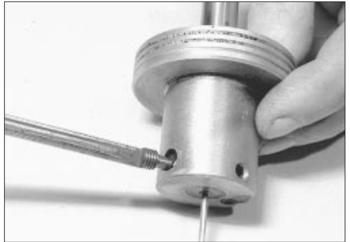
13.35b . . . and secure with the retaining screw
