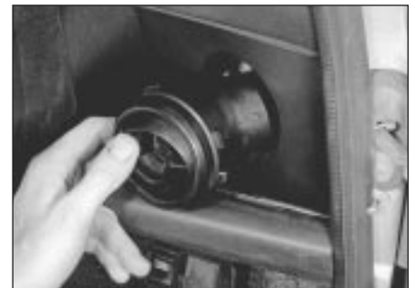
13.2 Turn the air vent anti-clockwise to remove
