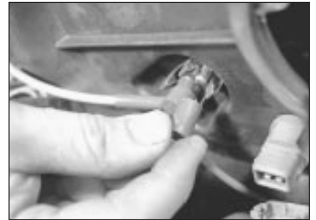
2.2b . . . and the thermac valve vacuum pipe
