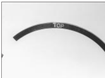
16.3 Piston ring identification markings
