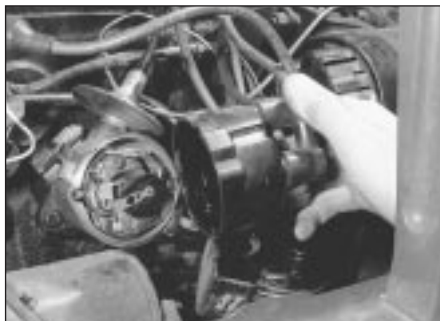
5.1 Removing the distributor cap
