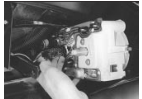
15.28b ... and the multiplug connector, then lift away the instrument panel
