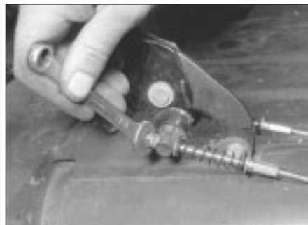
21.3 Remove the handbrake cable adjusting nuts
