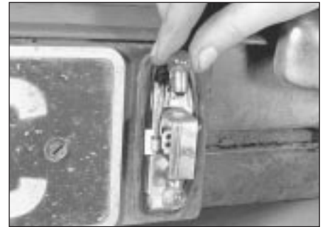
5.48 . . . and remove the bulbs by turning them anti-clockwise
