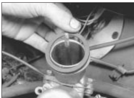
2.2b Recover the sealing ring
