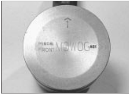
11.19 Identification markings on the piston crown
