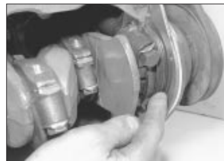
5.25 Fitting a new front oil seal . . .
