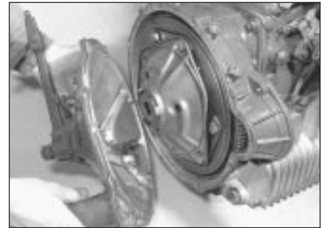
5.3 Removing the flywheel housing cover
