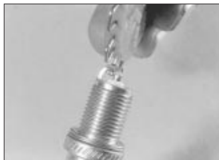
33.11 Adjusting a spark plug electrode gap
