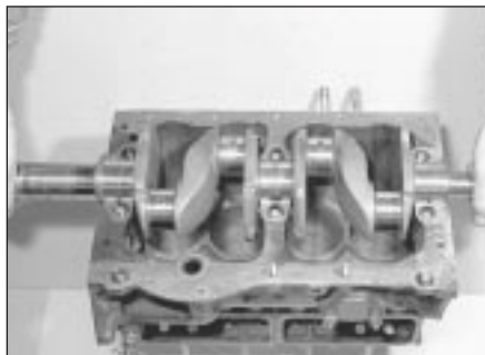
12.10 Carefully lift out the crankshaft
