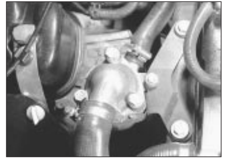
5.3b Thermostat housing and radiator upper mounting bracket (later 1275 cc models)
