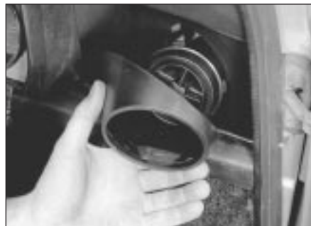
13.1b ... and lift away the binnacle
