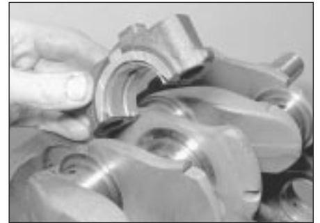
12.8 Main bearing cap with thrustwashers in position
