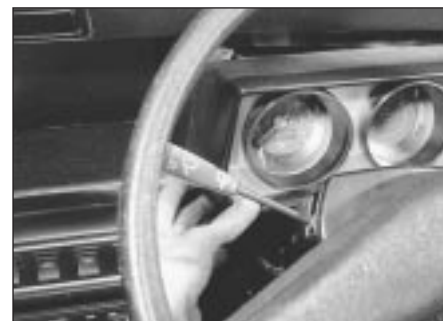
15.25 Remove the instrument cluster nacelle
