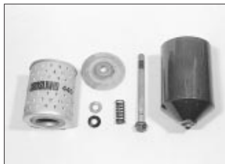
13.9 Components of the cartridge type oil filter
