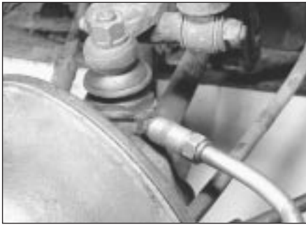
16.1a Lubricating the swivel hub upper grease nipple . . .
