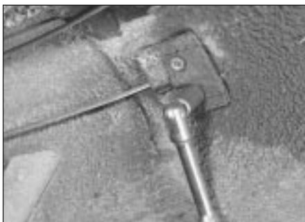
21.5a Hold the cable guide retaining nuts from below . . .
