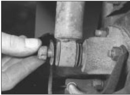
17.3 Remove the shock absorber lower ...
