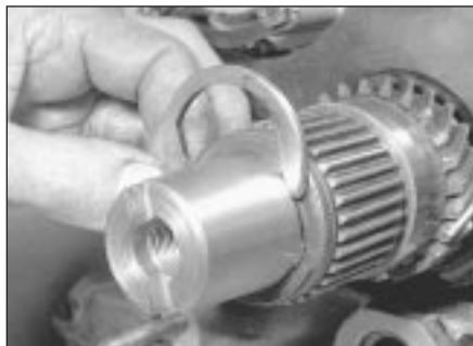
5.31b . . . and the C-shaped washer
