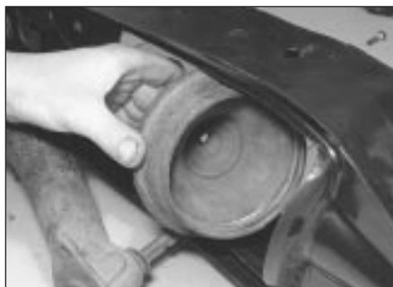
15.4 . . . and rubber cone spring
