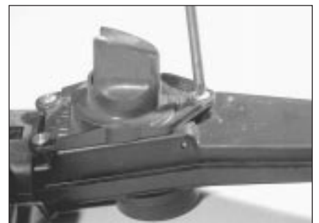
3.12 Removing the air cleaner intake duct adapter
