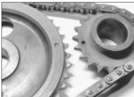
5.22a Timing dots on sprockets aligned with chain fitted
