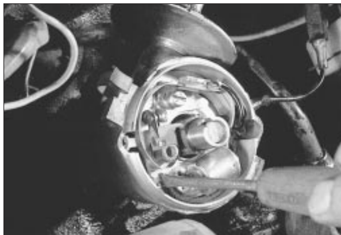
5.7 Adjusting the contact breaker points
