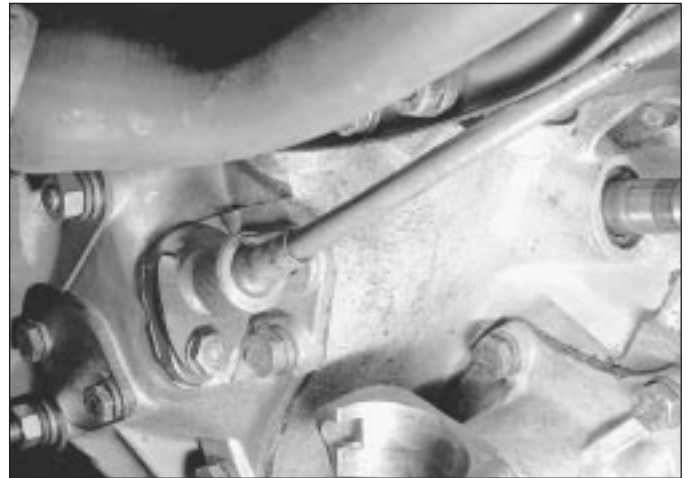
3.44b . . . until sufficient clearance exists to disconnect the speedometer cable
