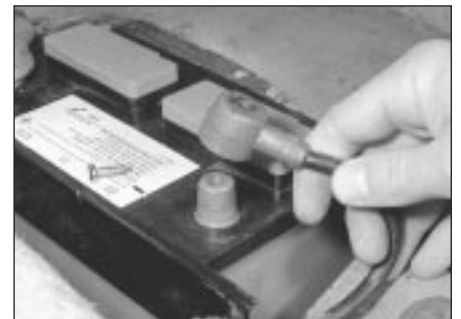
4.2 Disconnecting the battery negative lead (Saloon model shown)
