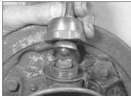
5.12a Refit the ball-pin and nut ...
