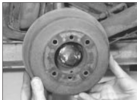
4.3 . . . and withdraw the drum
