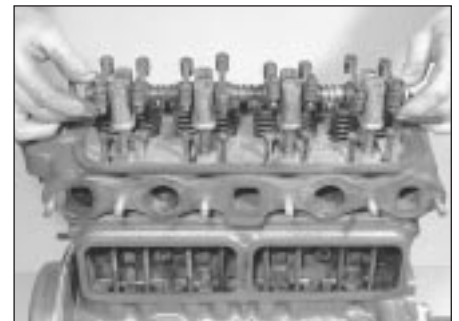
7.15b . . . then lift off the rocker shaft assembly
