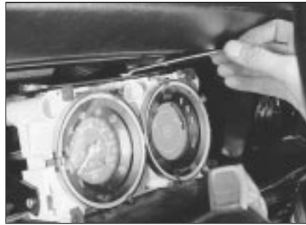
15.27b ... and upper retaining screws
