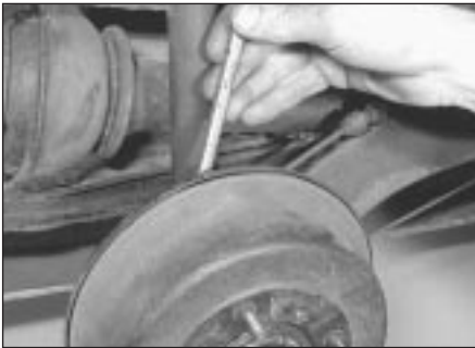
3.9 Adjusting the rear brakes
