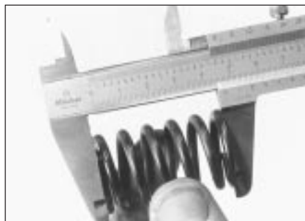
8.25 Measuring valve spring free length
