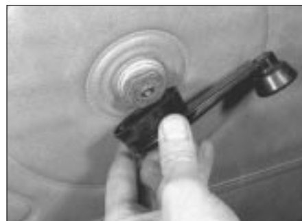
6.2b . . . and the window regulator handle
