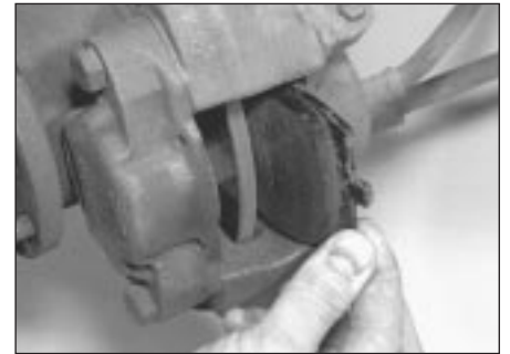
7.3b . . . then withdraw the two brake pads
