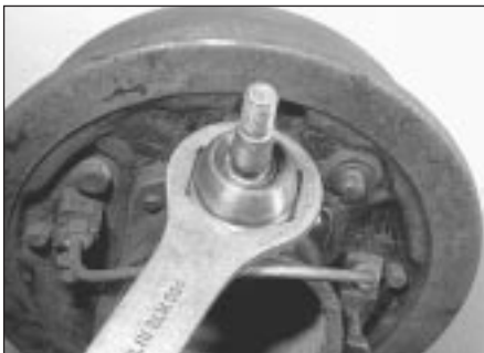
5.12c ... and fully tighten the nut
